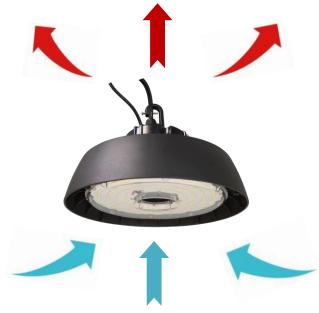
Radiator adopts ADC12 aluminum integrated die-casting molding, which has small thermal resistance. The center of the lamp is designed with a unique convection hole to form a chimney convection hear dissipation, which can make the lamps get a better cooling effect in harsh environments.
